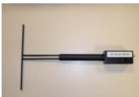
Figure 1 – Satimo COMOSAR Validation Dipole
