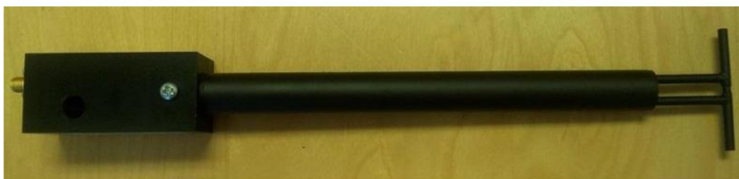
Figure 1 – MVG COMOSAR Validation Dipole
