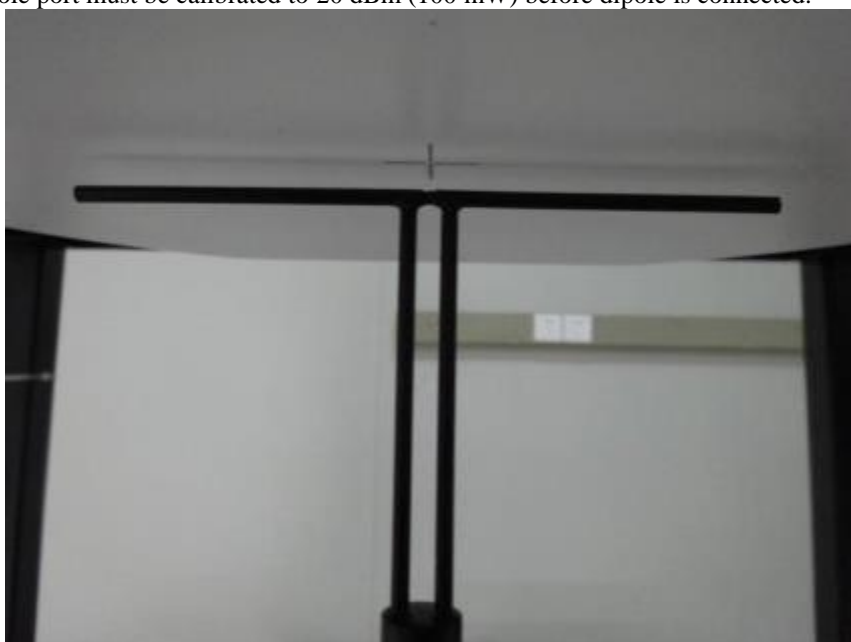
Photo of Dipole Setup
