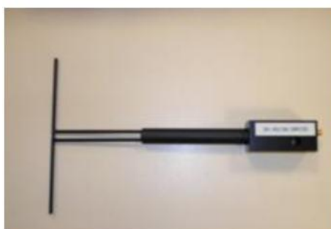
Figure 1 – Satimo COMOSAR Validation Dipole
