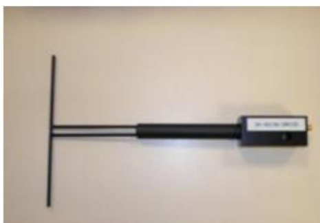
Figure 1 – Satimo COMOSAR Validation Dipole
