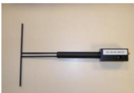
Figure 1 – Satimo COMOSAR Validation Dipole
